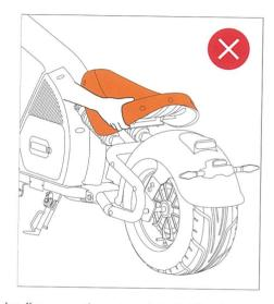
2. Please handle or move the motorcycle by holding the frame with one hand as shown in the above picture. 2. soft materials and can be deformed or damaged under the action of the strong force, and thus don't apply the strong force when handling or moving the motorcycle.
