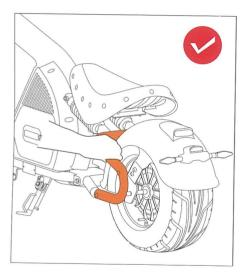
1. Please handle or move the motorcycle by holding the frame with one hand as shown in the above picture.
