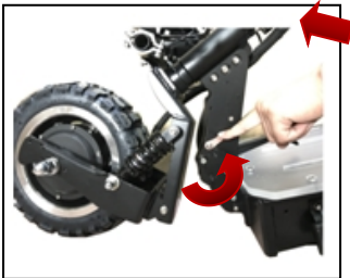
Step 1 Push down the folding Lock, and Push back the Pole At the same time
