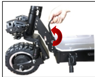
Step 2 Push back the Safety Lock
