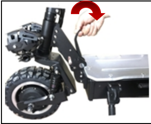
Step 1 Pull down the safety Lock
